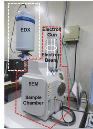
Figure 3 External View of SEM/EDX Equipment
