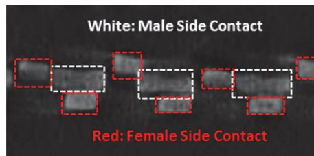
Figure 20 CT Scan of Contact Shorting
