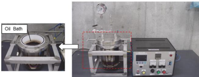
Figure 6 Sulfuration Accelerated Aging Test Equipment
