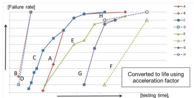
Figure 15 Accelerated Sulfuration Resistance Test
