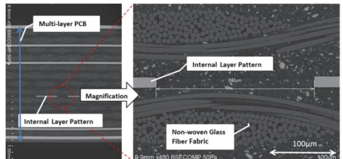
Figure 7 Cross Section of Multi-layer PC Board
