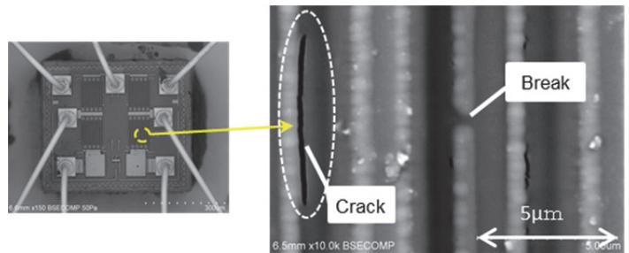
Figure 12 ESD Break in IC Chip (SEM)
