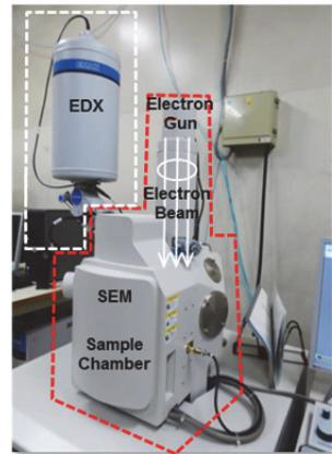
Figure 3 External View of SEM/EDX Equipment
