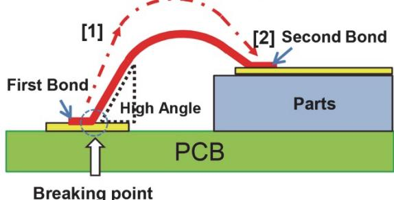
Figure 11 Schematic of Faulty Lot
