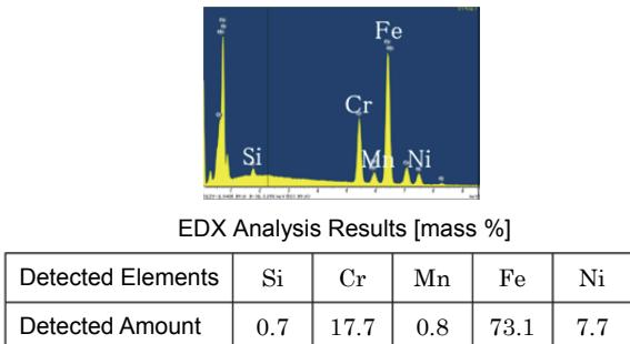
Figure 5 EDX Analysis of SUS304 Stainless Material
