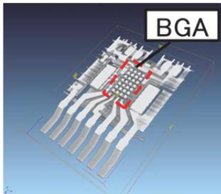
Figure 18 Magnified X-ray CT Scan
