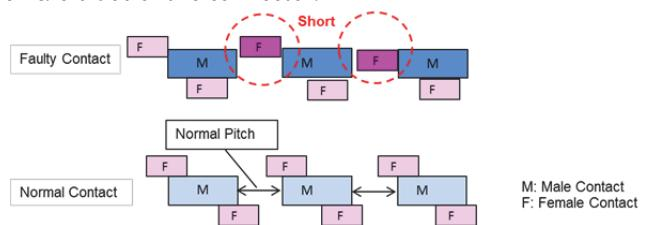
Figure 21 Faulty Contact Conditions
