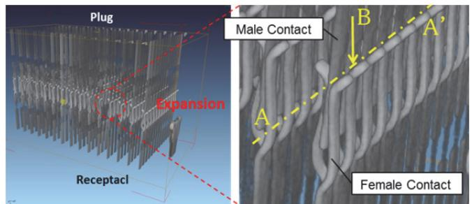
Figure 19 Connector (Fitting Condition) CT Scan Stereoscopic Image
