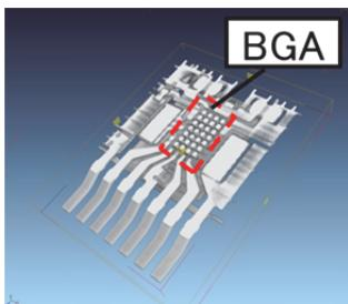
Figure 18 Magnified X-ray CT Scan
