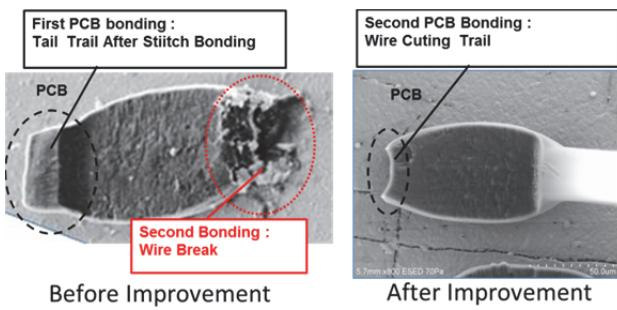
Figure 9 Magnified View of Wire Bonding
