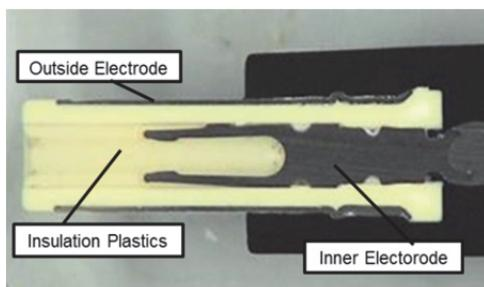
Figure 17 DC Plug Internal Structure
