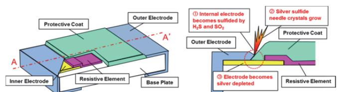
Figure 13 Cross-Section of Thick-Film Chip Resistor
