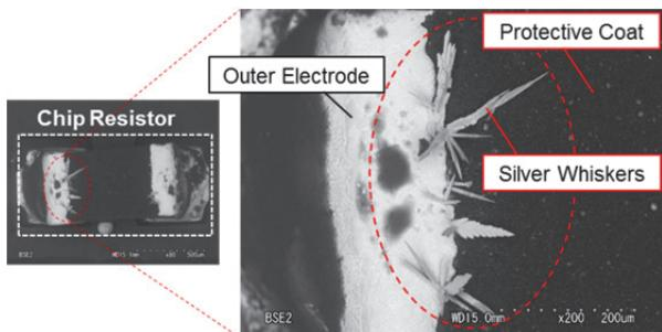
Figure 14 Silver Sulfide Crystal Formation (SEM)
