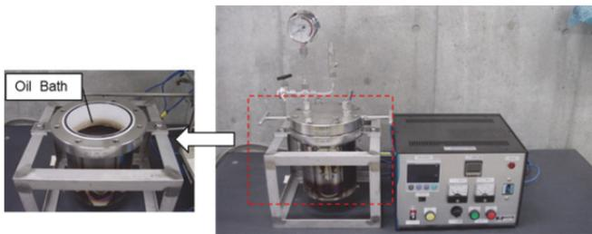
Figure 6 Sulfuration Accelerated Aging Test Equipment
