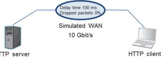
Figure 14 Test Configuration 1 (without TCP acceleration)
