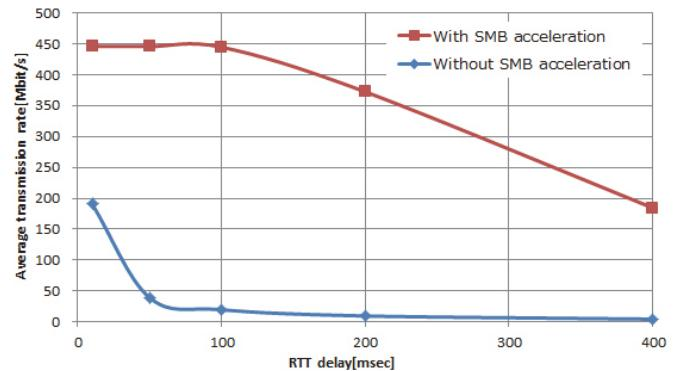
Figure 18 Throughput with SMB Protocol
