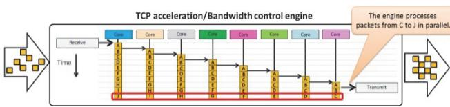
Figure 7 Parallel Processing by Multicore Processor
