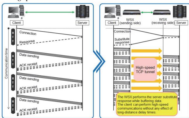
Figure 6 Typical TCP Response Sequence
