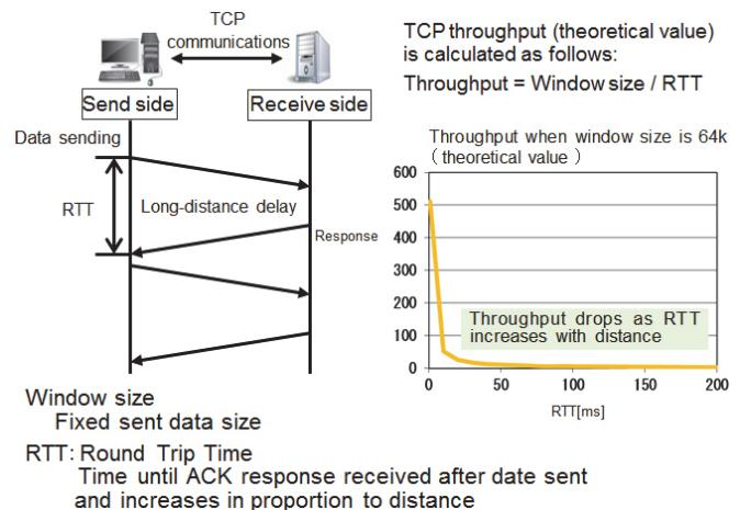
Figure 1 Delay Mechanism at TCP Communications
