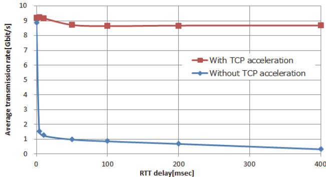
Figure 16 High-Speed TCP Throughput
