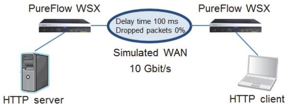
Figure 15 Test Configuration 2 (with TCP acceleration)
