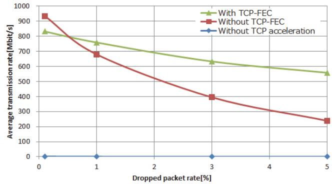
Figure 17 Throughput with Dropped Packets (RTT 100 ms)
