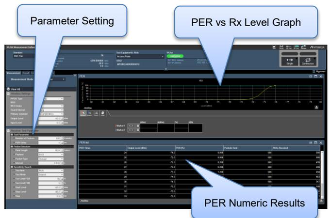
Figure 7 WLAN Rx Measurement Window
