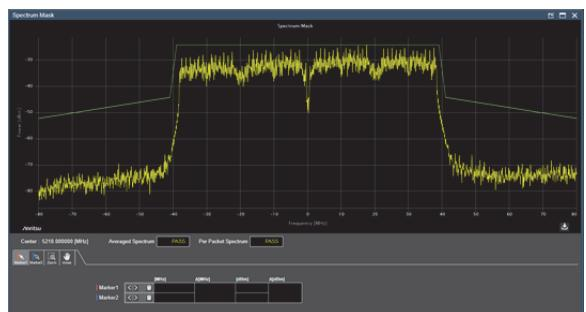
Figure 10 Spectrum Mask Results Window
