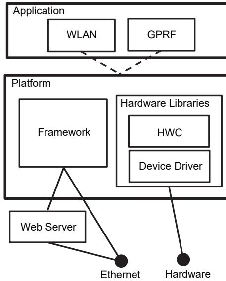
Figure 3 Main CPU Software Structure
