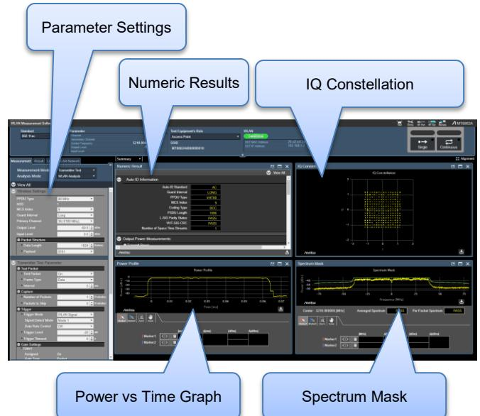
Figure 6 WLAN Tx Measurement Window
