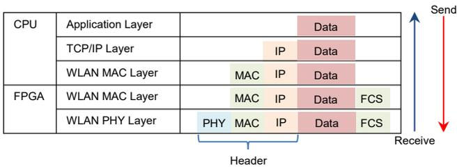
Figure 5 Processing for Each Layer
