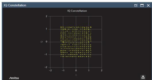
Figure 9 IQ Constellation Window (256QAM)
