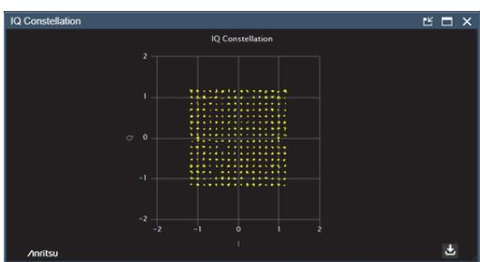
Figure 9 IQ Constellation Window (256QAM)
