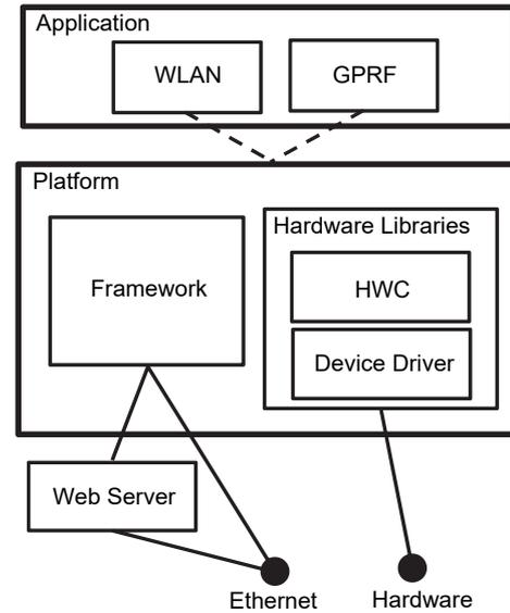
Figure 3 Main CPU Software Structure
