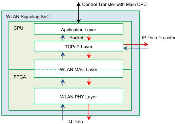
Figure 4 WLAN Signaling SoC Function Blocks
