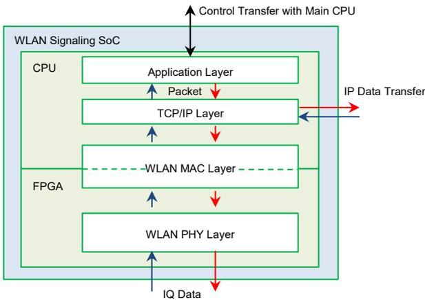
Figure 4 WLAN Signaling SoC Function Blocks
