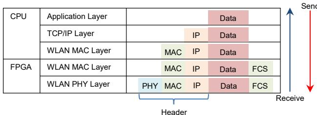
Figure 5 Processing for Each Layer
