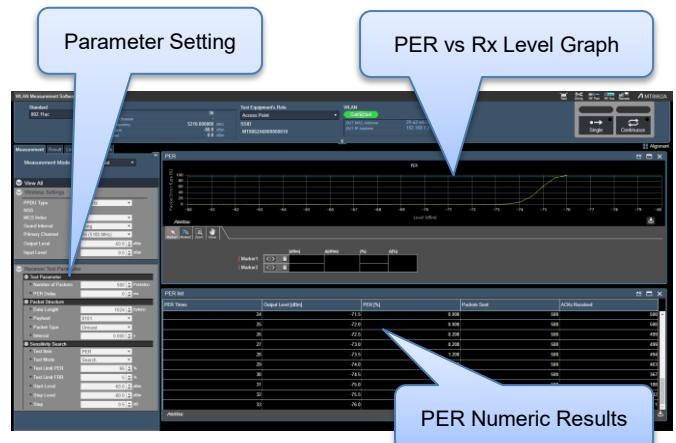
Figure 7 WLAN Rx Measurement Window
