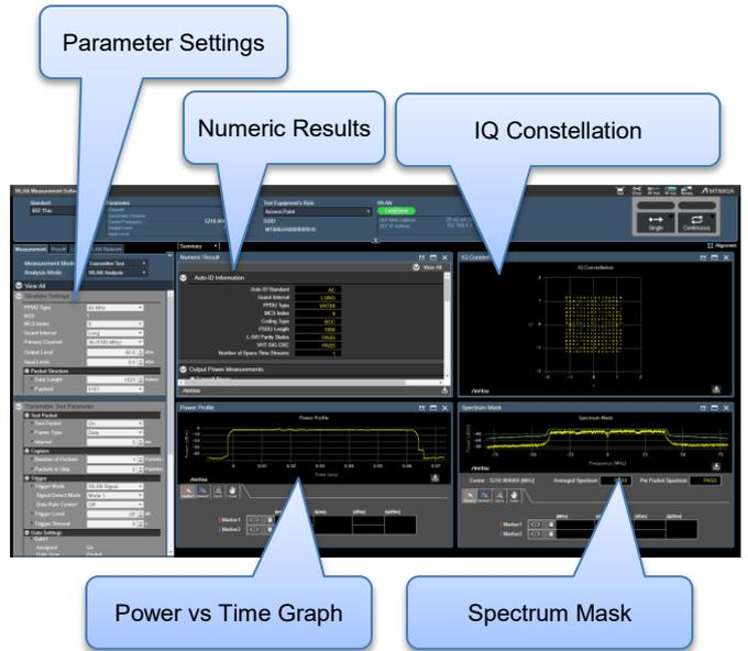
Figure 6 WLAN Tx Measurement Window
