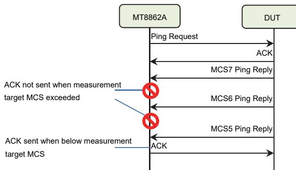
Figure 14 Tx Data Rate Control
