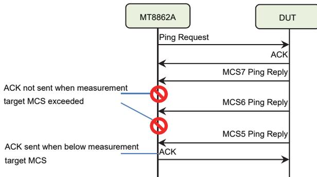
Figure 14 Tx Data Rate Control
