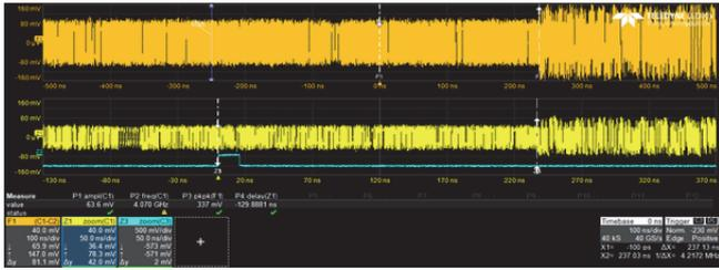
Figure 15 Link Equalization Output Waveform
