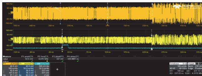
Figure 15 Link Equalization Output Waveform
