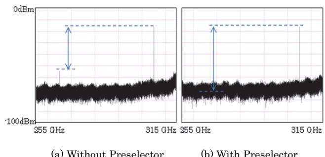
Figure 13 Spectrum at Multiple Response Generation
