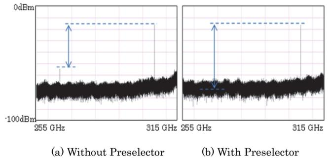
Figure 13 Spectrum at Multiple Response Generation
