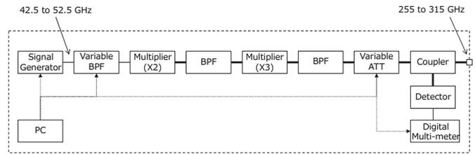
Figure 6 300-GHz Band Signal Generator Blocks
