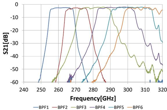
Figure 5 Filter-Bank Frequency Characteristics
