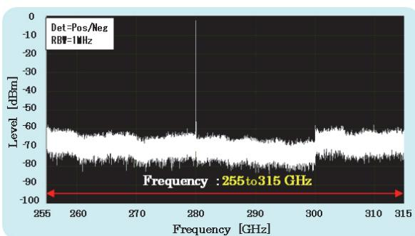
Figure 11 Spectrum (at input of 280-GHz CW signal)
