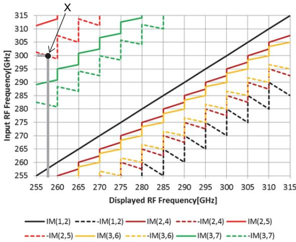
Figure 2 300-GHz Band Spectrum Measurement System Spurious
