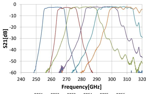
Figure 5 Filter-Bank Frequency Characteristics
