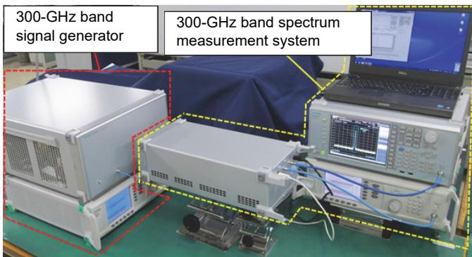
Figure 10 External Appearance of 300-GHz Band Spectrum Measurement System and 300-GHz Signal Generator
