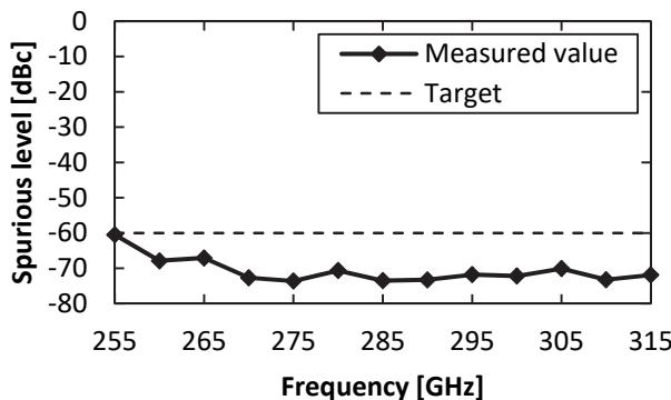
Figure 8 Spurious Characteristics of 300-GHz Band Signal Generator
