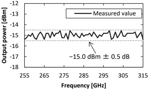
Figure 7 Output Power Characteristics of 300-GHz Band Signal Generator
