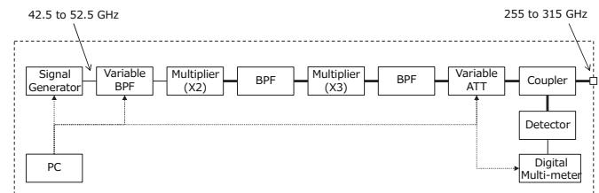
Figure 6 300-GHz Band Signal Generator Blocks
