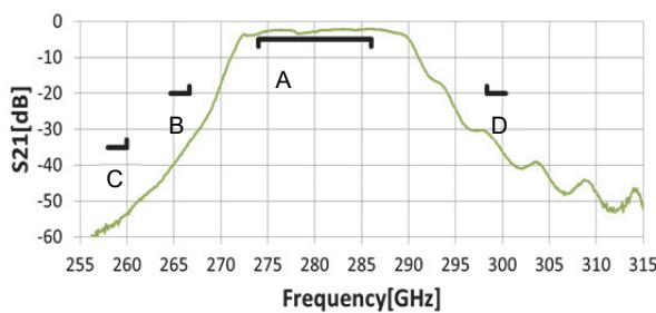
Figure 4 BPF Frequency Characteristics for Band 5 and Band 6
