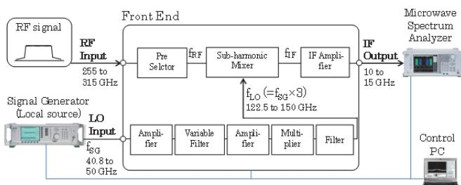
Figure 1 300-GHz Band Spectrum Measurement System Blocks
