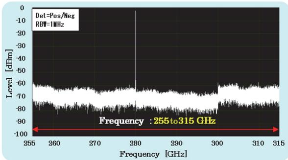
Figure 11 Spectrum (at input of 280-GHz CW signal)
