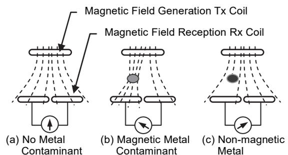
Figure 4 Magnetic and Non-Magnetic Metals in AC Magnetic Field
