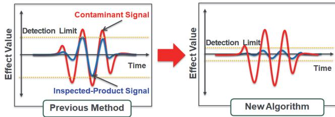
Figure 7 Concept of new algorithm
