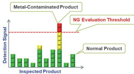
Figure 2 Metal Detector Sensing Image
