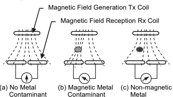
Figure 4 Magnetic and Non-Magnetic Metals in AC Magnetic Field
