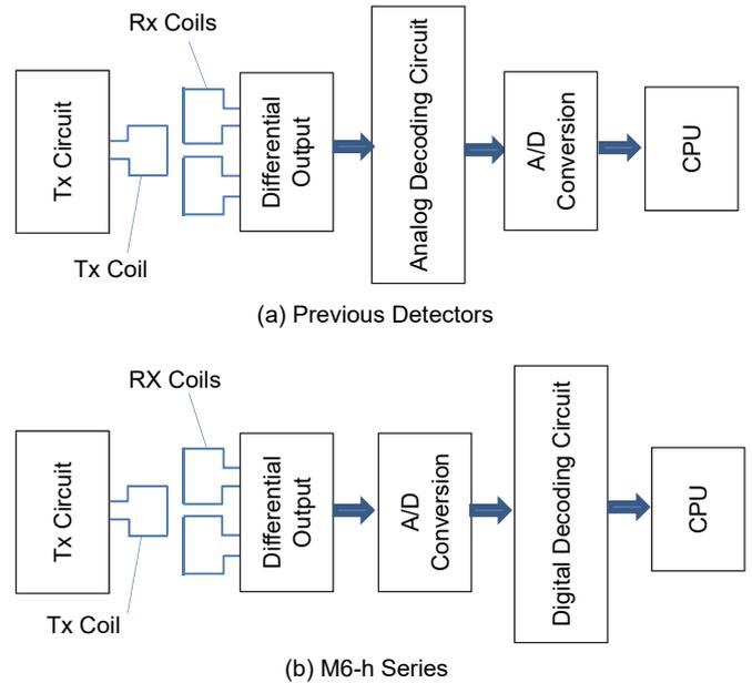
Figure 6 Metal Detector Sensor Circuit
