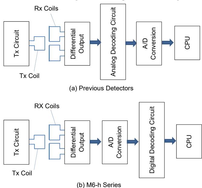
Figure 6 Metal Detector Sensor Circuit
