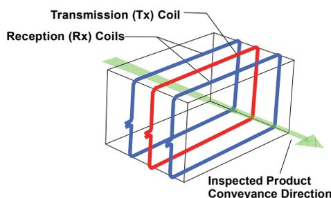
Figure 3 Detection Head Coil
