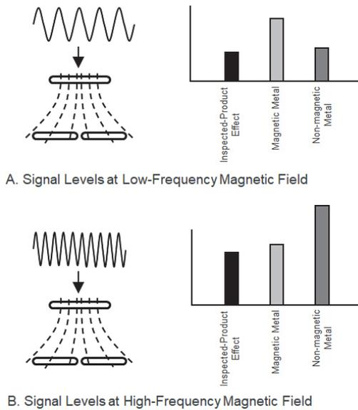
Figure 5 Relationship between Magnetic Frequency and Signal Level
