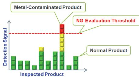
Figure 2 Metal Detector Sensing Image
