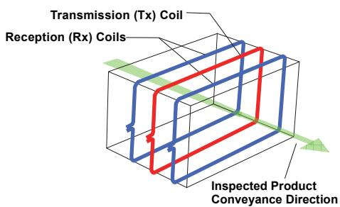
Figure 3 Detection Head Coil
