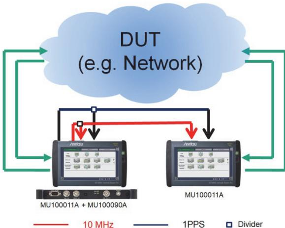
Figure 10 One-Way Latency Measurement System with Two MT1000A Units
