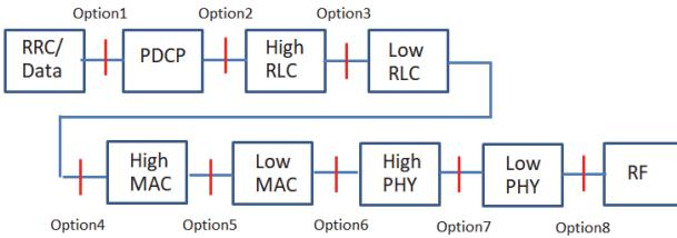
Figure 1 Division of Functions Between CU and DU<sup>3)</sup>
