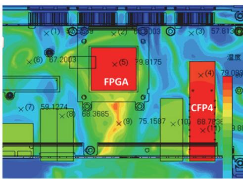
Figure 6 Example of Thermal Simulation Results
