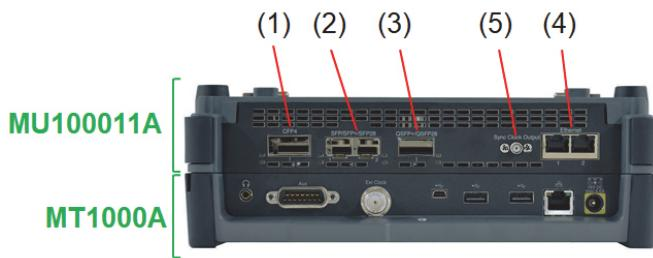
(1) CFP4, (2) SFP28, (3) QSFP28, (4) RJ45, (5) Sync Clock Output
