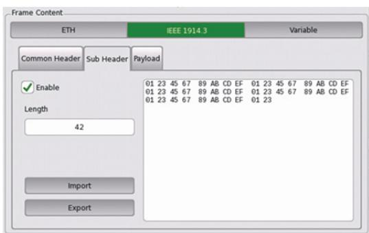
Figure 9 RoE Tx Frame Setting Screen
