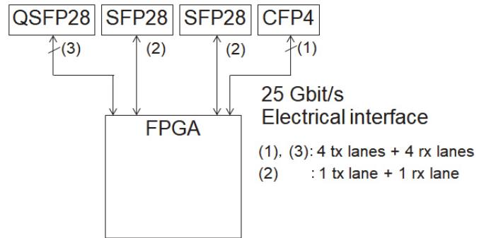
Figure 3 25 Gbit/s Electrical I/F Circuit Block Diagram
