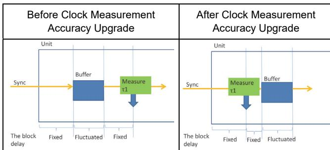
Figure 13 Comparison of Clock Measurement Accuracy Before and After Upgrade
