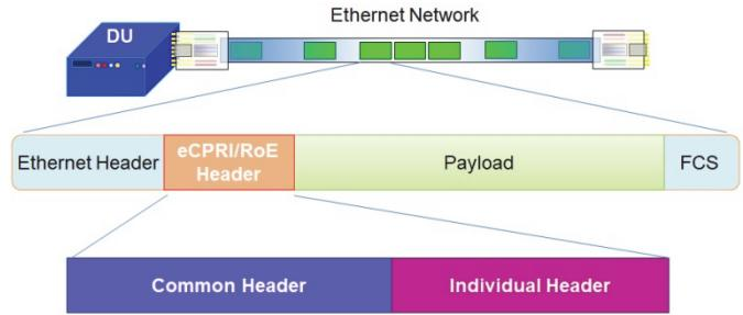
Figure 7 eCPRI/RoE Frame Structure
