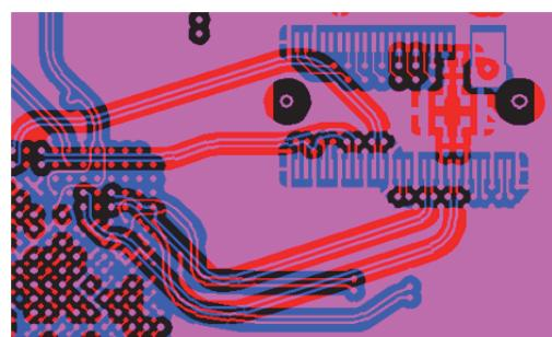
Figure 4 PC Board Wiring Pattern to CFP4 Connector
