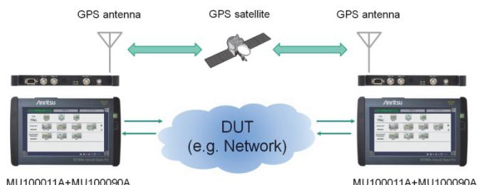
Figure 11 Far-End One-Way Latency Measurement System
