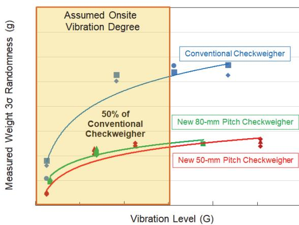
Figure 9 Improved Vibration Damping
