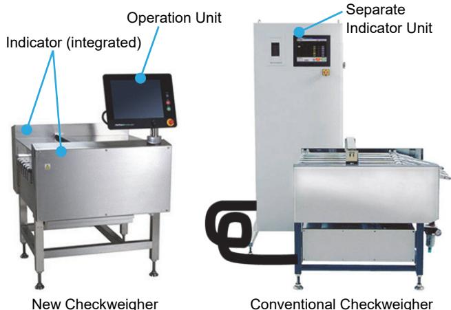
Figure 10 External Views of New and Conventional Checkweighers
