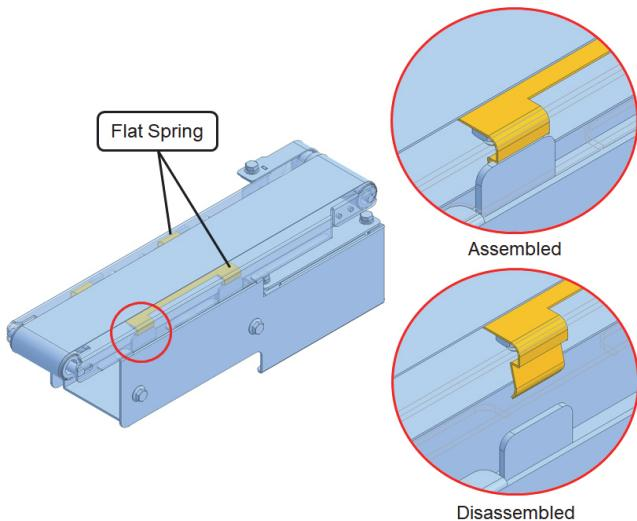
Figure 14 Tool-free Assembly/Disassembly
