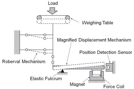
Figure 4 Force Balance Weighing Mechanism
