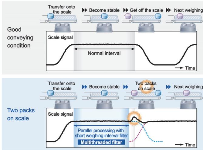
Figure 11 SMF Measurement Principle
