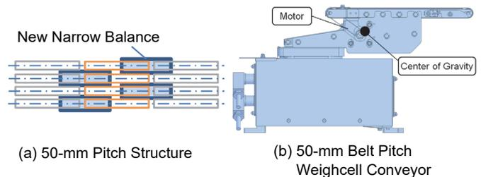
Figure 7 50-mm Belt Pitch Support
