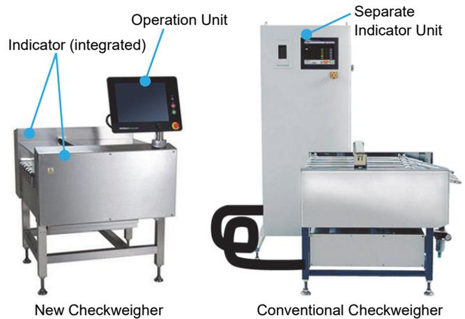
Figure 10 External Views of New and Conventional Checkweighers
