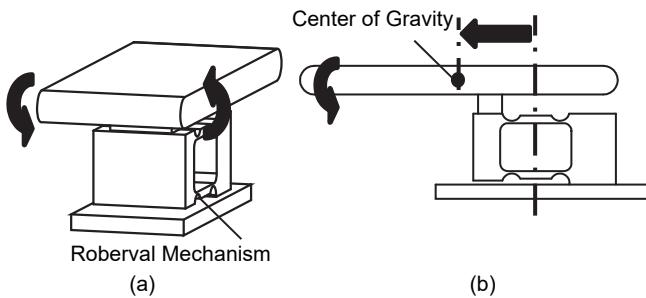
Figure 5 Weighcell Roberval Structure Side Rigidity
