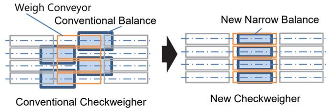
Figure 6 Weighcell Arrangement (80-mm Belt Pitch)
