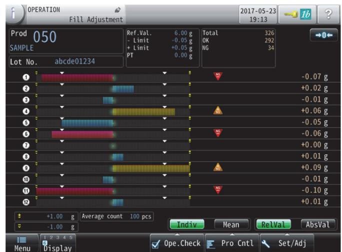
Figure 12 Fill Adjustment Screen
