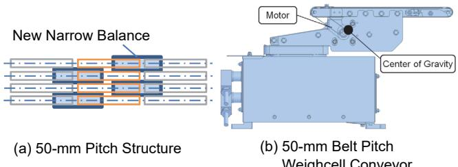
Figure 7 50-mm Belt Pitch Support
