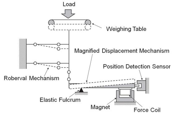
Figure 4 Force Balance Weighing Mechanism
