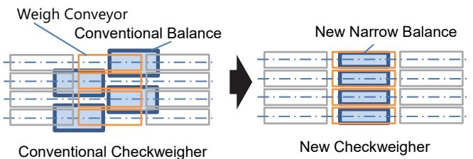
Figure 6 Weighcell Arrangement (80-mm Belt Pitch)
