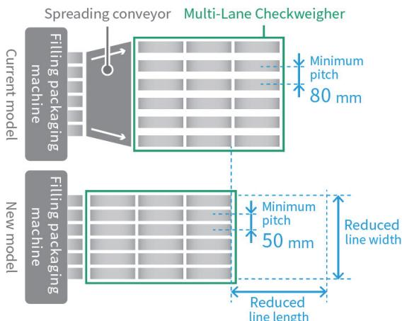
Figure 8 Space Saving by Reducing Belt Pitch
