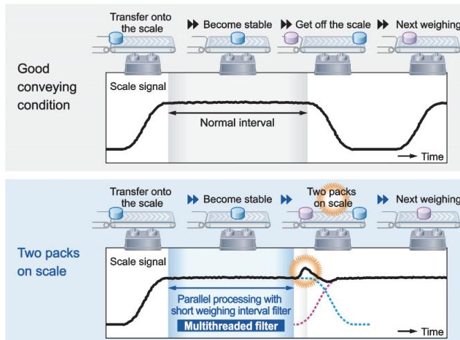
Figure 11 SMF Measurement Principle
