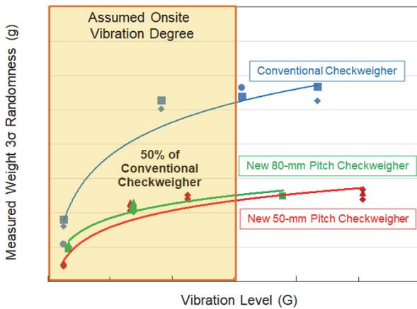
Figure 9 Improved Vibration Damping
