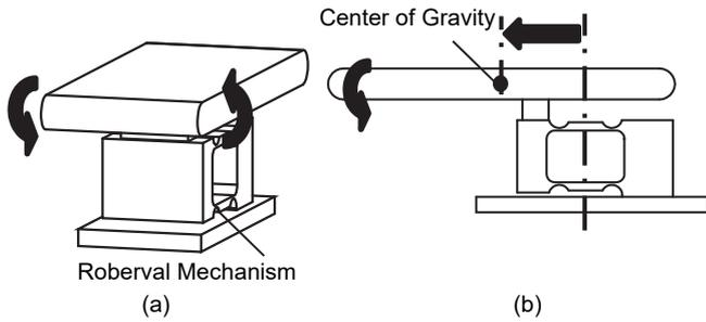
Figure 5 Weighcell Roberval Structure Side Rigidity
