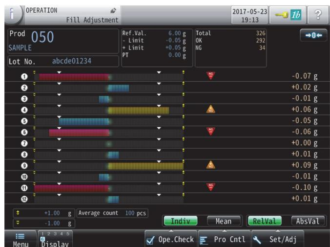
Figure 12 Fill Adjustment Screen
