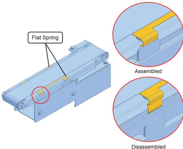
Figure 14 Tool-free Assembly/Disassembly
