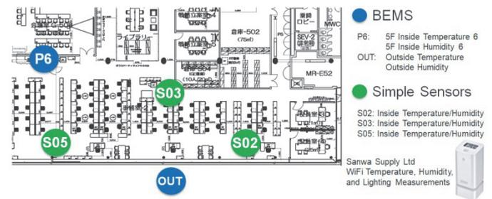
Figure 8 Locations of Simple Temperature and Humidity Sensors
