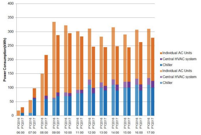
Figure 12 Changes in AC Power Consumption Over Time
