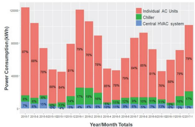
Figure 2 Power Usage by AC Type
