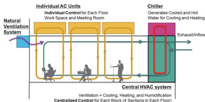
Figure 1 Air Conditioning System Configuration
