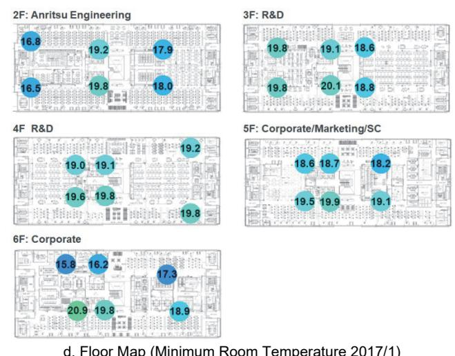
Figure 4 Visualization of Temperature and Humidity by Floor
