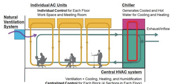
Figure 1 Air Conditioning System Configuration
