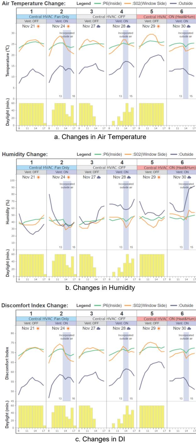
Figure 9 Changes in Temperature, Humidity, and Discomfort Index During Test Period
