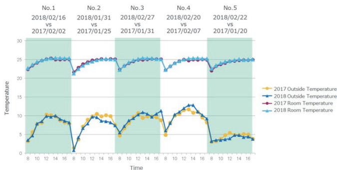
Figure 11 Trend in Outside Temperature and Room Temperature for Compared Target Days
