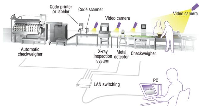
Figure 5 QUICCA System Configuration Example
