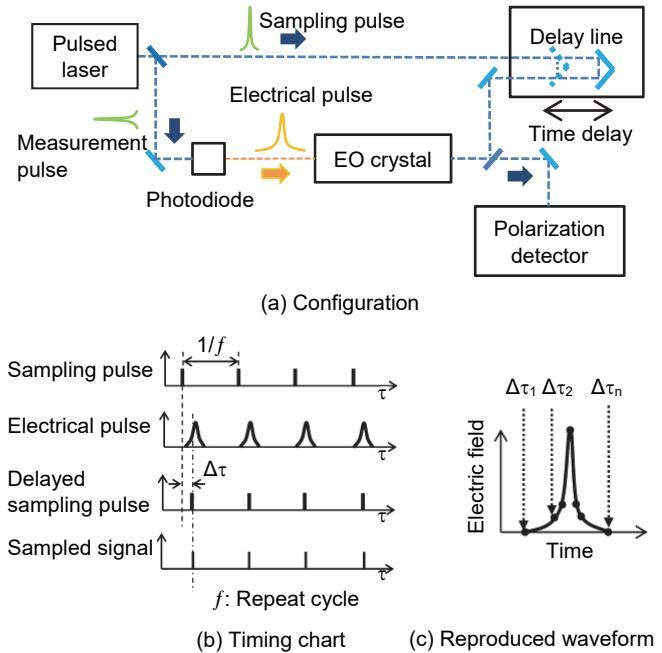
Figure 3 Electrical Pulse Waveform Measurement using EO Sampling
