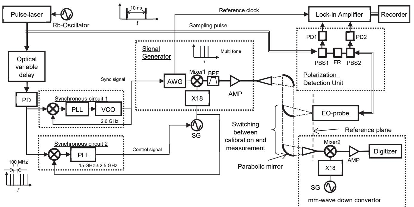
Figure 5 Test Setup for Measuring mmWave 3-Tone Signal using EO Sampling
