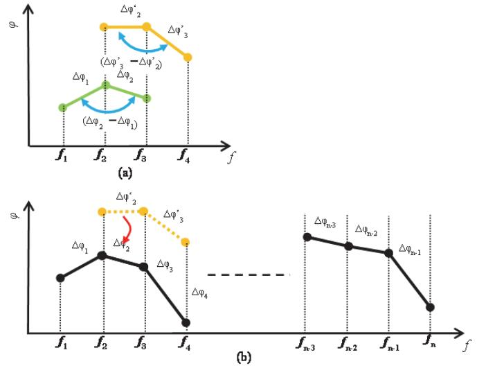
Figure 4 Phase Connection at Acquisition of Frequency Characteristics using Multitone Signal
