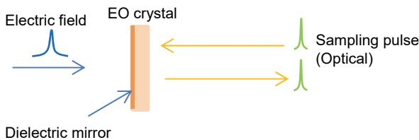
Figure 2 Structure of Field Strength Detector using EO Crystal
