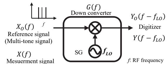
Figure 1 Principles of Phase-Characteristics Calibration
