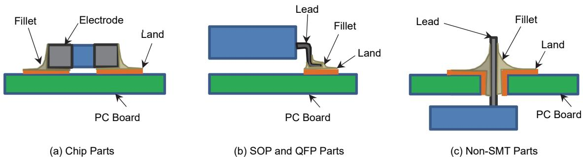
Figure 2 Examples of Normal Fillet Shapes
