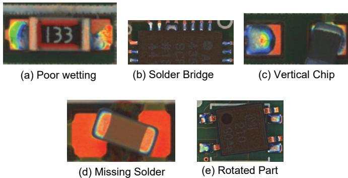
Figure 3 Examples of SMT Mounting Faults
