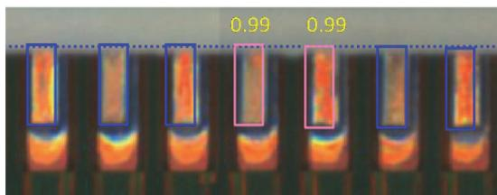
Figure 12 Example of Mis-detection (Missed Fail Location)
