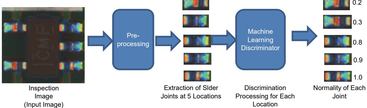
Figure 5 Discrimination Procedure using Machine Learning
