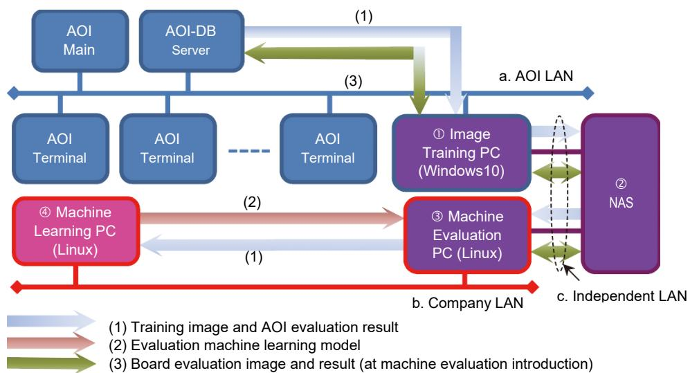
Figure 4 Image Acquisition System Configuration
