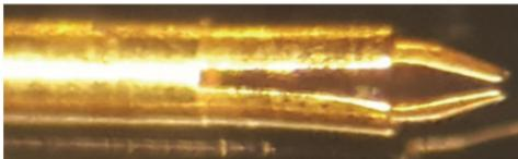
Figure 4 A formed 0.261 mm dia. slotted male contact pin
