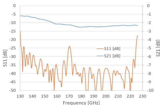
Figure 13 Reflection and Transmission response of Anritsu's 35WR5G 0.6-mm coax-to-WR5 adapter
