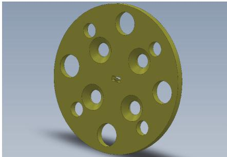
Figure 8 Zoomed-out view of 0.6-mm Flange to WR5 in-line shim transition
