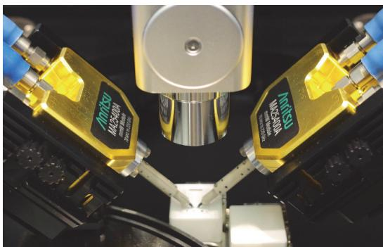
Figure 16 Two-port wafer probe measurement using MPI flanged coaxial wafer probes direct connected to Anritsu's MA25400A reflectometer modules.
