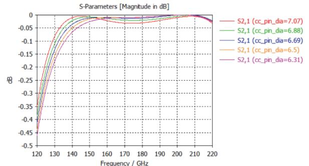
Figure 11 Parametric sweep of  $|S_{21}|$  vs. Frequency, by varying diameter of solid pin inside a 7.1 mil dia. hole
