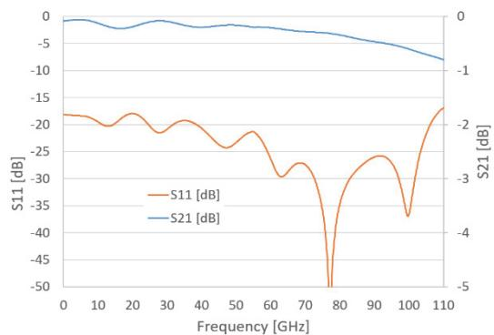
Figure 15 Reflection and Transmission response of Anritsu's 33WG50 1-mm (W1) coax-to-0.6 mm Flange adapter
