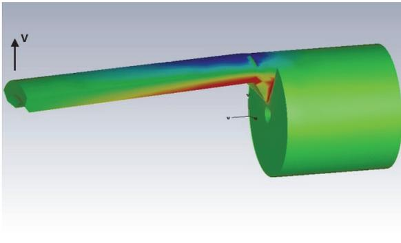
Figure 2 Strain analysis on a single finger of a 1.85 mm (V) four-slot slotted contact with outward force at end of finger in V-axis direction.
