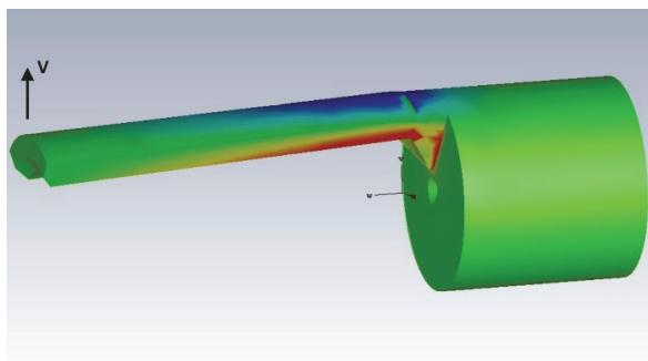
Figure 2 Strain analysis on a single finger of a 1.85 mm (V) four-slot slotted contact with outward force at end of finger in V-axis direction.
