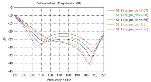
Figure 10 Parametric sweep of  $|S_{11}|$  vs. Frequency, by varying diameter of solid pin inside a 7.1 mil dia. hole
