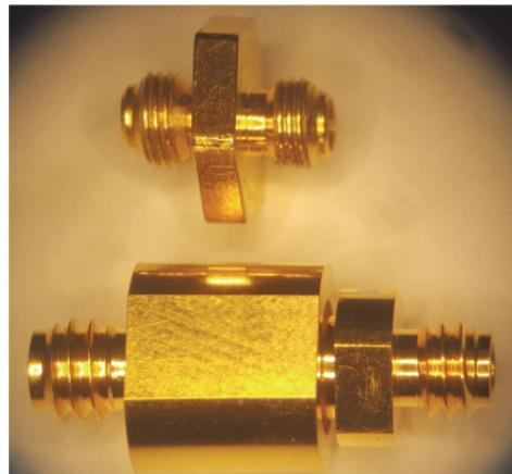
Figure 3 Length comparison between Anritsu 33.8F.8F50 0.8-mm F-F adapter (top) and Anritsu 33WFWF50 1-mm (W1) adapter (bottom)
