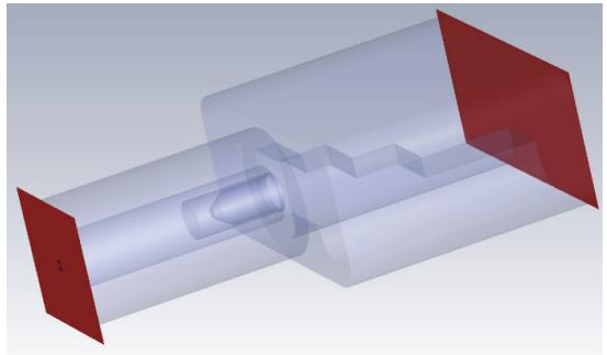
Figure 9 3D EM model of 0.6-mm coax-to-WR5 Waveguide transition with integrated pin
