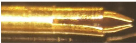
Figure 4 A formed 0.261 mm dia. slotted male contact pin
