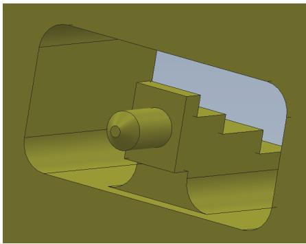
Figure 6 Integrated pin 0.6-mm Flange to WR5 in-line shim transition
