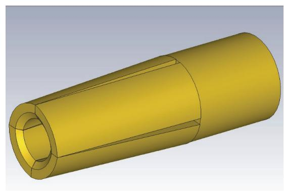
Figure 1 1.85 mm (V) four-slot slotted contact
