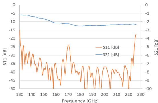
Figure 13 Reflection and Transmission response of Anritsu's 35WR5G 0.6-mm coax-to-WR5 adapter
