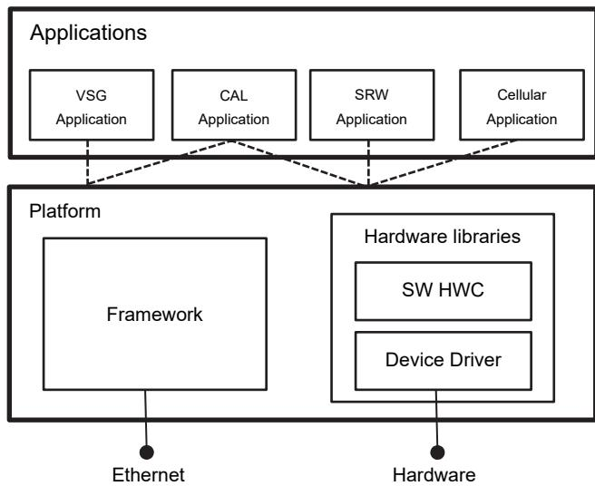
Figure 3 MU887002A Software Structure
