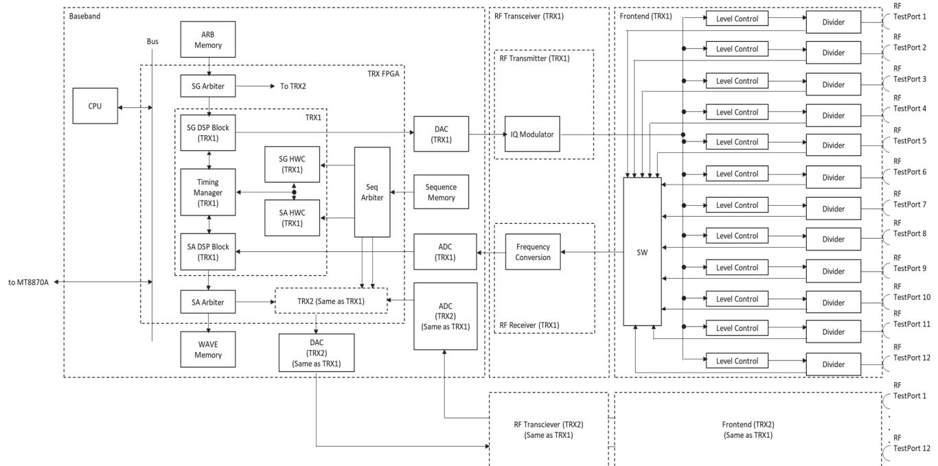
Figure 2 MU887002A Block Diagram
