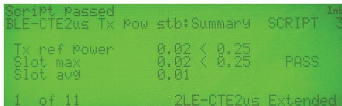
Figure 12 Tx Power Stability Measurement Screen (Reference period, Slot typical values)
