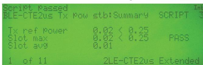
Figure 12 Tx Power Stability Measurement Screen
