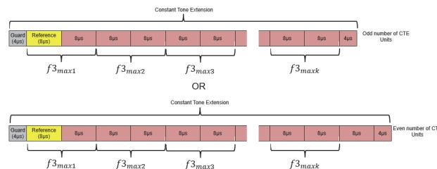
Figure 10 Constant Tone Extension Frequency Drift
