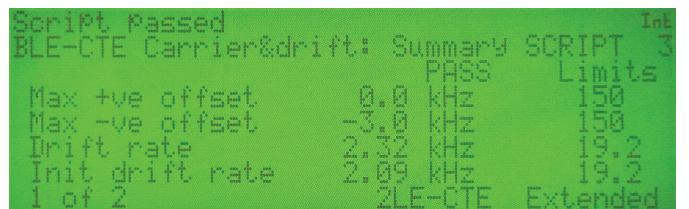
Figure 11 Carrier Frequency Offset and Drift Measurement Screen
