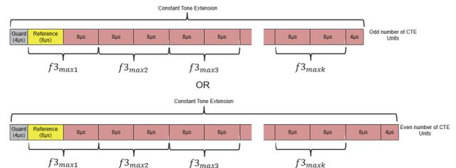
Figure 10 Constant Tone Extension Frequency Drift
