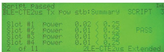
Figure 13 Tx Power Stability Measurement Screen (Each Slot)
