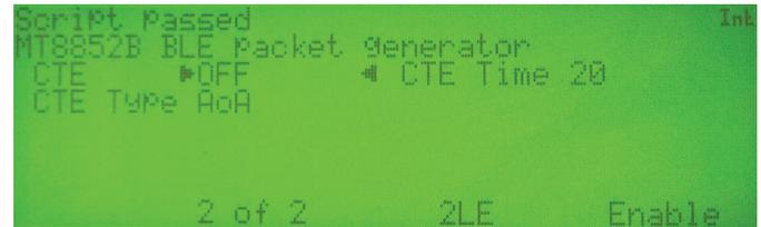
Figure 14 BLE Packet Generator Setting Screen (CTE Settings)
