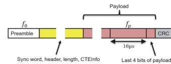
Figure 9 Constant Tone Extension Reference Frequency ( $f_0, f_p$ )
