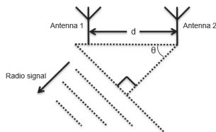
Figure 5 Departure Direction Detection
