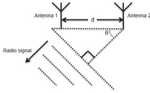
Figure 5 Departure Direction Detection
