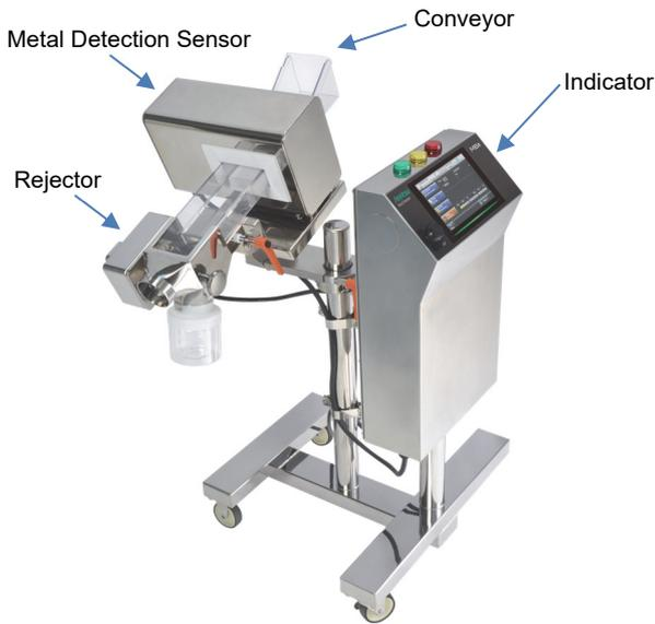
Figure 2 Structure of Metal Detector
