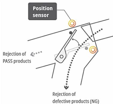
Figure 10 Rejector Position Sensor
