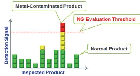
Figure 3 Metal Detector Sensing Image
