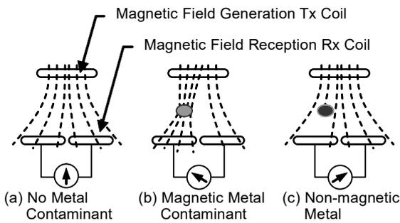
Figure 5 Magnetic and Non-Magnetic Metals in AC Magnetic Field
