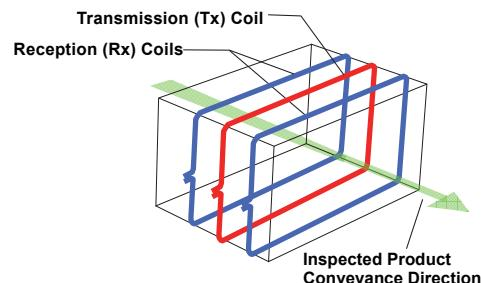
Figure 4 Detection Head Coil
