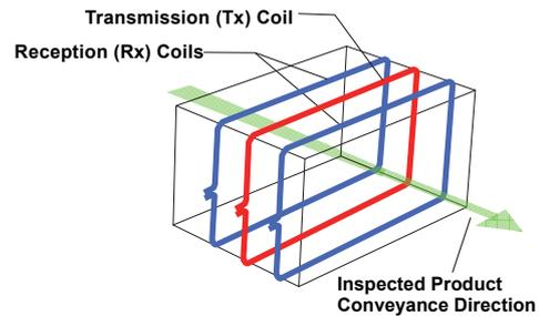
Figure 4 Detection Head Coil
