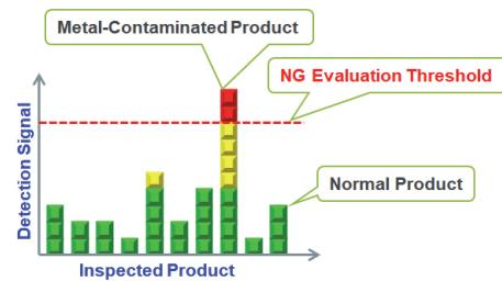
Figure 3 Metal Detector Sensing Image
