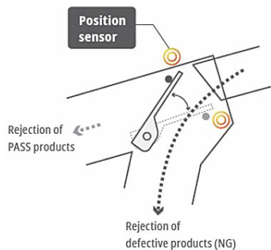
Figure 10 Rejector Position Sensor
