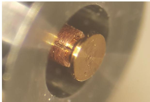
Figure 10 Capacitively compensated watermelon seed pin installed into the backside of a 1.85 mm (V) connector
