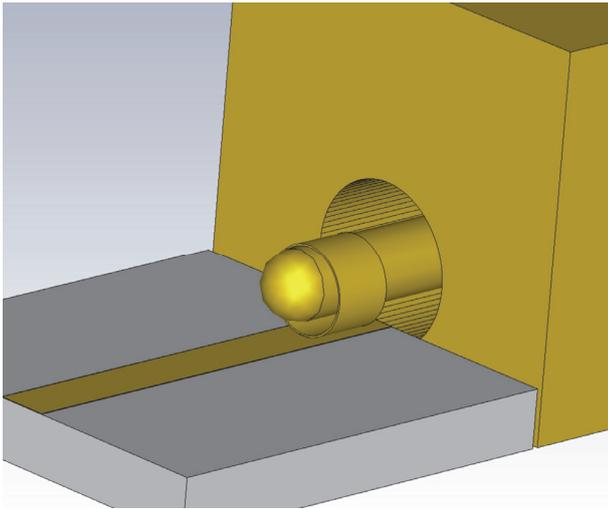
Figure 1 Backside pin overlap on 10-mil thick Alumina using gold ribbon-wrap
