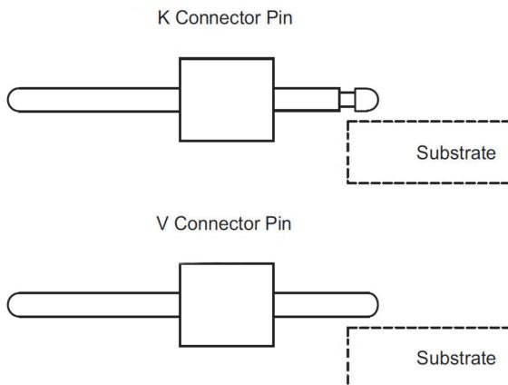
Figure 3 K and V pressure contact pins of Anritsu 3680 Universal Test Fixture (UTF)
