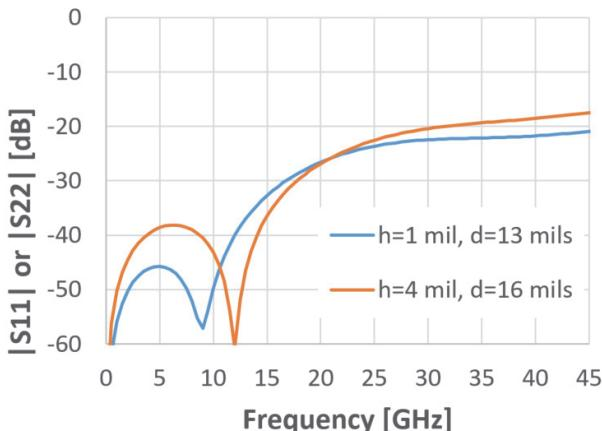
Figure 2 Parametric reflection response of gold ribbon-wrap model
