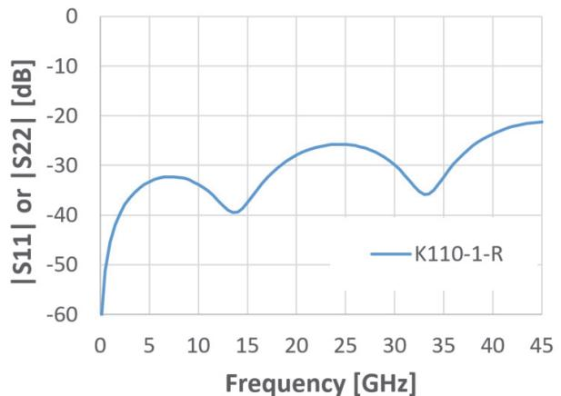
Figure 5 Typical reflection response of Sliding Contact model
