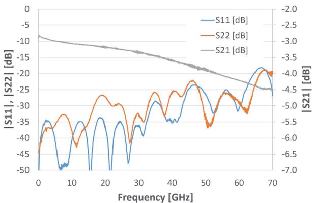
Figure 12 Response of a 1.85 mm (V) coaxial 3-dB attenuator assembly using Shielded Suspended Substrate Stripline circuit and watermelon seed axial contact
