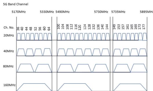
Figure 3 5-GHz band Channel Arrangement
