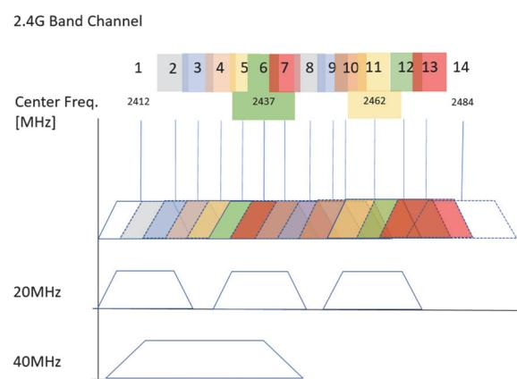
Figure 2 2.4-GHz band Channel Arrangement
