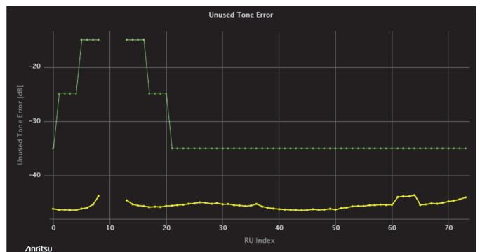
Figure 8 160-MHz Bandwidth Signal Unused Tone Error Measurement
