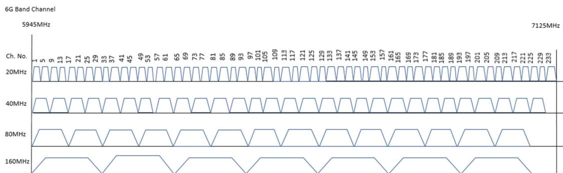
Figure 4 6-GHz band Channel Arrangement
