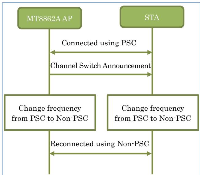
Figure 5 Non-PSC Channel Switch Sequence
