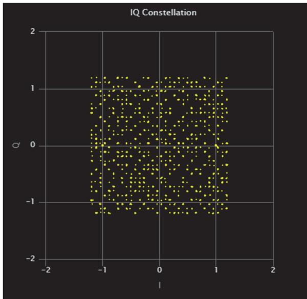
Figure 6 6-GHz band 1024QAM Constellation
