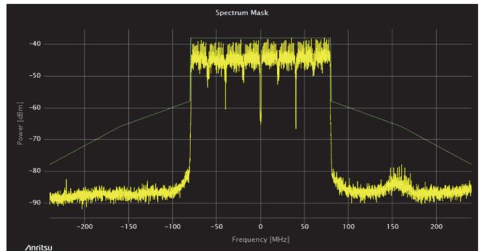
Figure 7 160-MHz Bandwidth Signal Spectrum Mask Measurement
