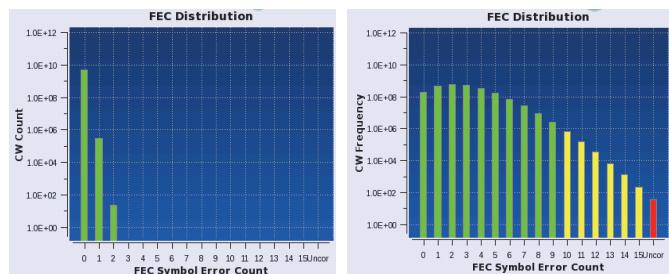
Figure 15 Symbol Error Rate Distribution
