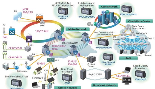
Figure 1 Network Communications Technologies and Speeds
