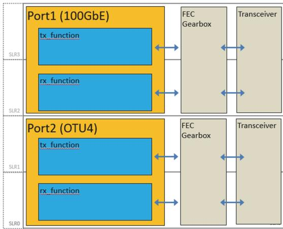
Figure 13 Partial Reconfiguration
