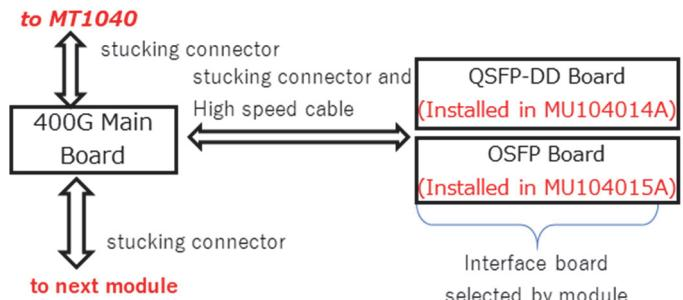
Figure 7 MU104014A/15A Block Diagram
