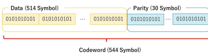
Figure 4 FEC Frame Structure
