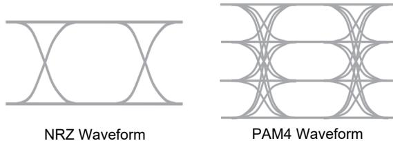
Figure 3 NRZ and PAM4 Waveforms
