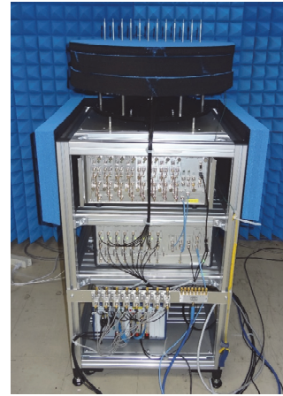
Figure 10 External View of Interference Monitoring Equipment (Sub-6 GHz Band Measurement)
