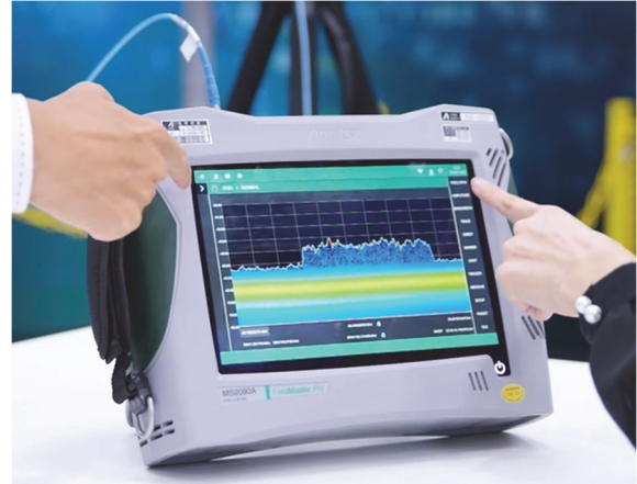
Figure 8 Visualizing 5G Waveform using Test Instrument
