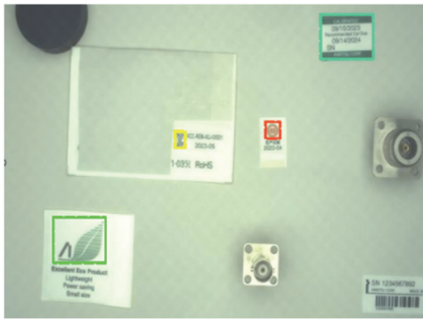
Figure 11 Using Deep Learning Function (Label Detection)
