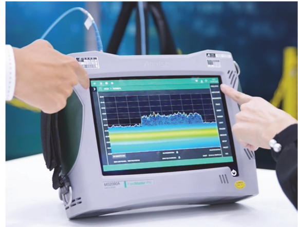
Figure 8 Visualizing 5G Waveform using Test Instrument
