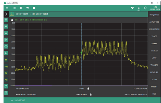
Figure 2 Single-side multitone generated signal showing 20 dBc image rejection before Calibration.
