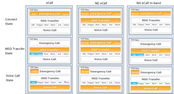
Figure 7 MX703330E PSAP Status Screens
