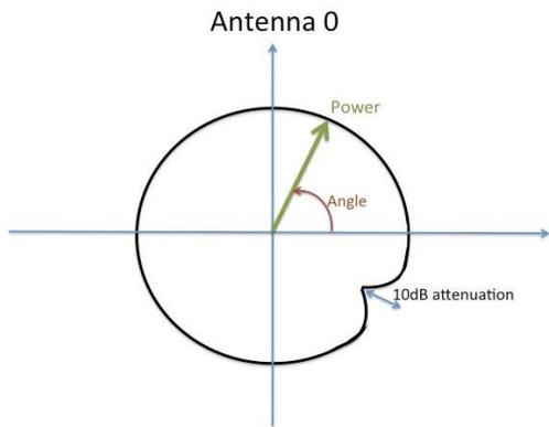
Figure 4: Ant0 received power during one rotation of the drone on itself
