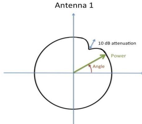
Figure 5: Ant1 received power during one rotation of the drone on itself
