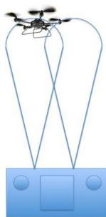
Figure 7: Remote controller antenna beams
