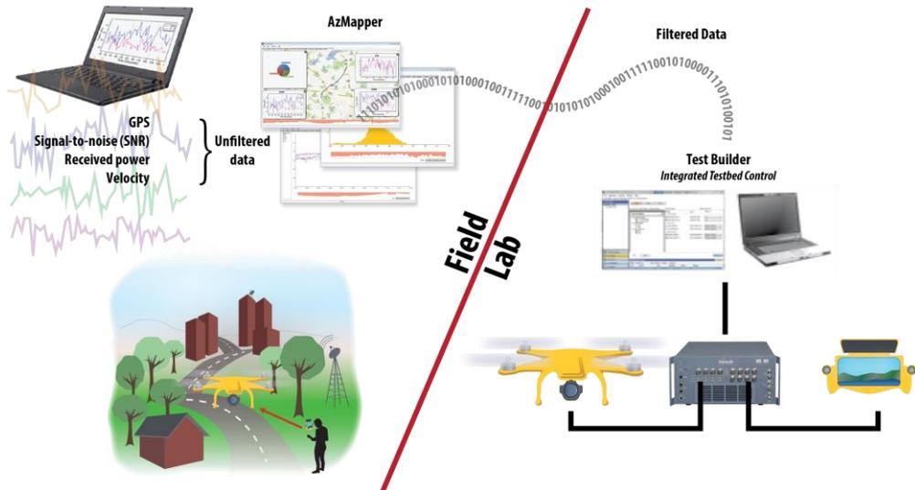
Figure 9: The Field-to-Lab process: Testing drones in the lab using recorded field conditions
