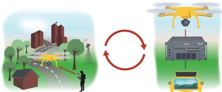
Figure 8: Using a channel emulator to replicate field conditions
