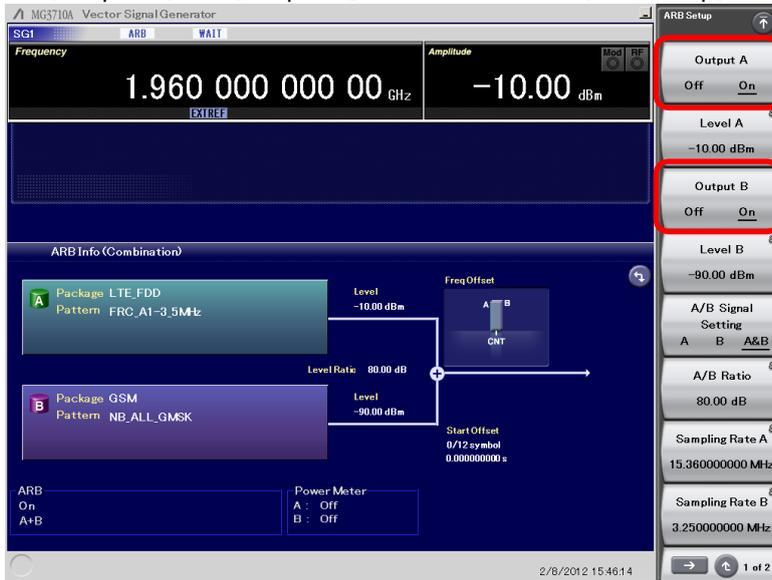
5. Set the level ratio of waveform memory A and B using [A/B Ratio] displayed by setting Mode to [ARB Setup]. In this example, this is 0 dB because no level ratio is appended. Set an appropriate level ratio matching the test contents.
