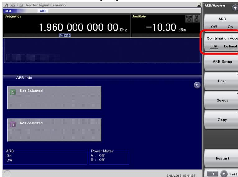
3. Click [Select] or Memory A, B shown on the screen to select the waveform pattern loaded into the waveform memory in step 1.
