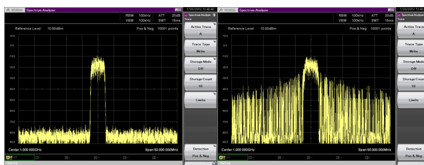
(a) Without clipping (b) With clipping Figure 14. Spectrum With and Without Clipping Effect
