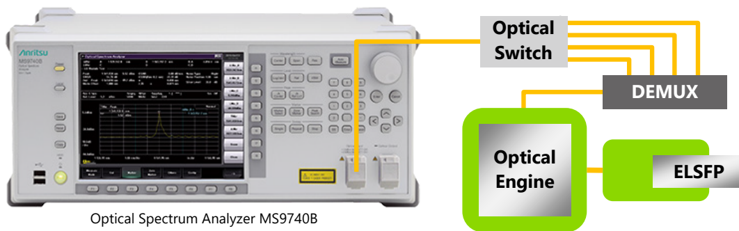
Figure 6 Optical Engine Optical Spectrum Test (400GBASE-FR4).
