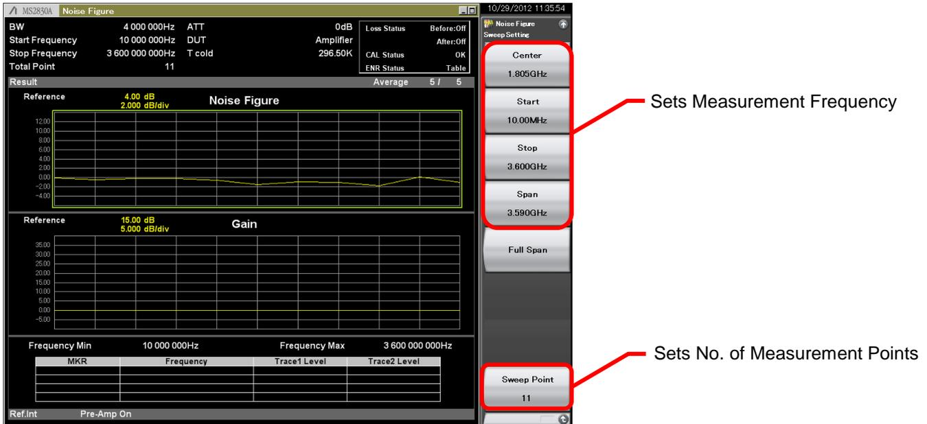
Fig. 3-7. Measurement frequency setting display
