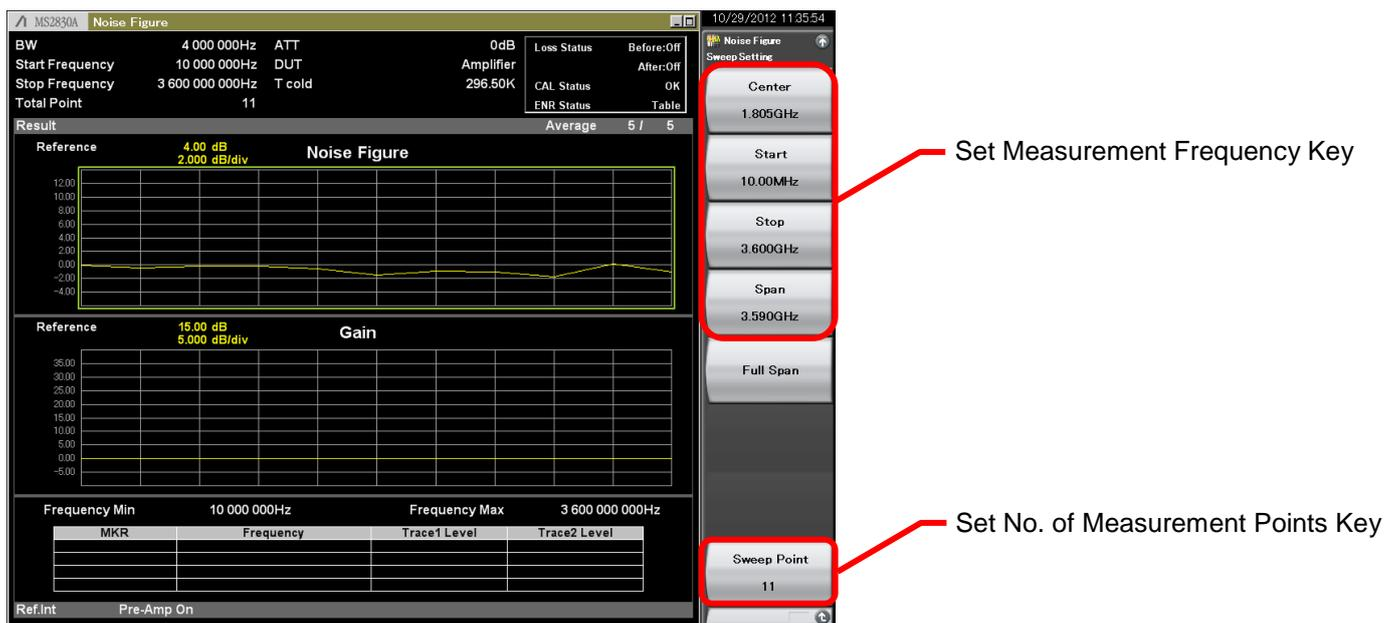
Fig. 4-16. Measurement Frequency Setting Display
