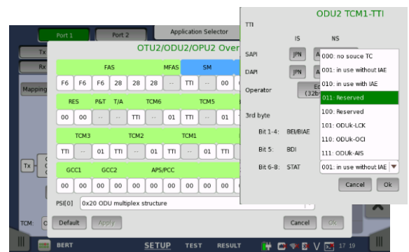
Figure 4. OTU transmitter Overhead
