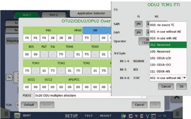
Figure 6 Edit Window for OTU/ODU/OPU Overhead
