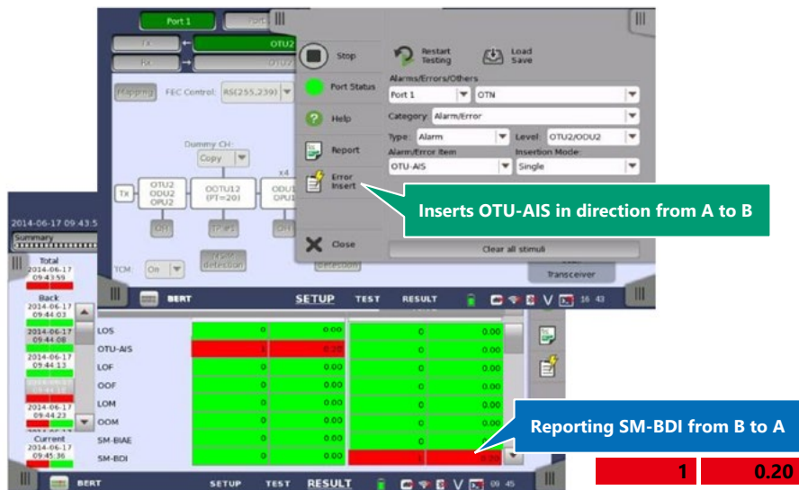
Figure 4 Alarm Injection and Detection in Pass-Through Mode BERT
