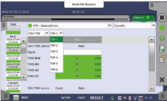
Figure 7 OTU TCM Receiver Alarms and Errors
