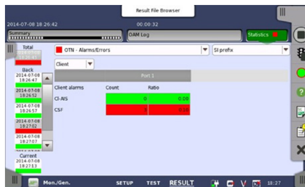
Figure 7 CSF Alarm Caused by Higher.
