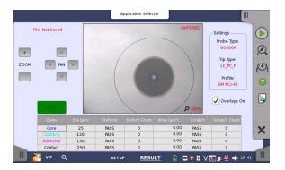
Endface after cleaning as seen with the VIP. The automatic pass/fail determination is made in accordance with the IEC61300-3-35 standard.
