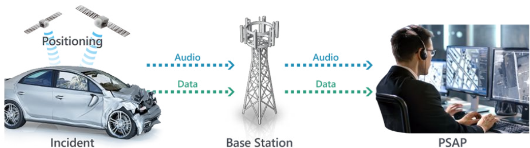
Figure 1 Emergency Call System.
