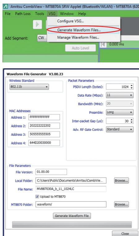
Figure 1. Waveform File Generator
