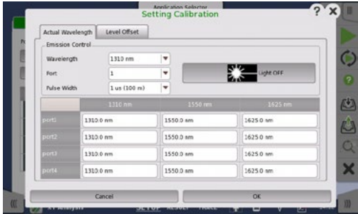
Setting of Measurement Optical Pulse and Input of Effective Center Wavelength
