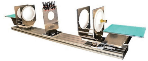
Figure 7 Appearance of Fixture for Free Space Method.
