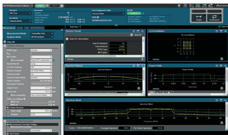
Example of Wi-Fi evaluation using Anritsu's MT8862A (Not actual nodoca™ evaluation data)
