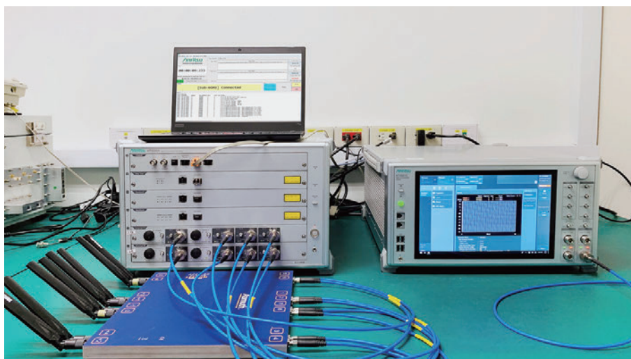
The MT8000A with Azimuth ACC-380 and Radio Communication Analyzer MT8821C were selected by USI-Taiwan 5G lab for RF measurement and protocol testing in the Sub-6 GHz NR band.
