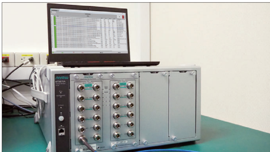
The Universal Wireless Test Set MT8870A supports RF testing for 5G Sub-6 GHz NR and other synchronous wireless communication tests.
