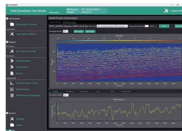
An example of the propagation characteristic analysis of captured radio signals using FST. The upper graph shows the analyzed delay spread profile. The lower graph indicates temporal variations in throughput.
