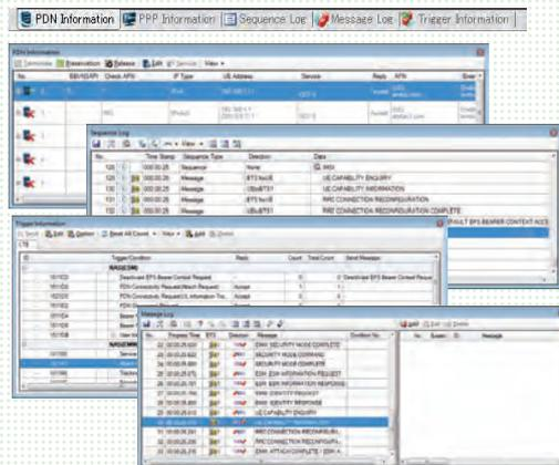
**5** Both base station parameters and packet communications can be controlled. Changes to status change parameters during testing are reflected immediately on-screen.
