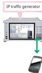
For the transmission and reception of the UE, use iPerf application which is widely used for throughput testing.
