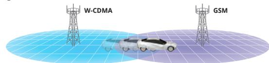
Figure shows the situation when the IVS switches from a 4G network connection used by Telematics services during driving to a 2G/3G network connection for eCall functions when an accident occurs. To emulate this type of test environment, the MD8475A and eCall Tester software perform the handover and CS Fallback switching tests in combination with the eCall function test.
