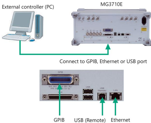
Remote control command is in common with the MG3710A and the MG3710E. Either select the SCPI mode command format defined by the SCPI Consortium, or select backwards compatible modes supporting earlier MG3700A, MS269xA, and MS2830A commands
