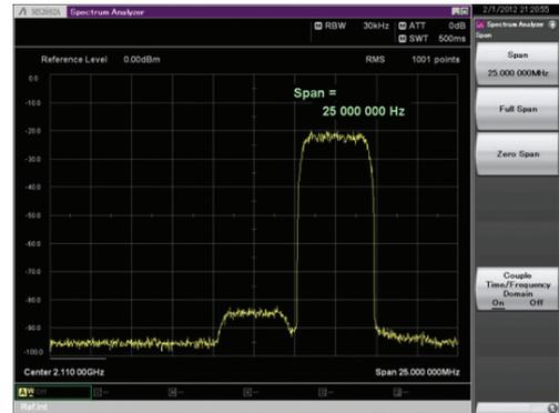
Spectrum of Wanted + Modulated Interference Signals
