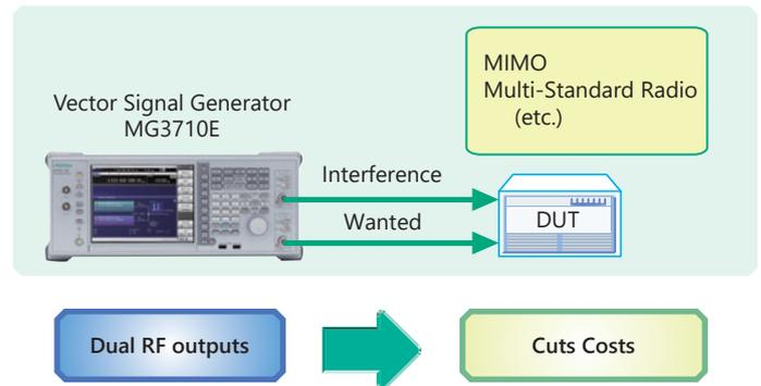
Two modulation signals can be output from one RF output using the baseband signal combine function (MG3710E-048/078). The level ratio (CN = 80 dB) and the frequency offset ( $\pm 80$  MHz max.) can be set as well. Tests using two modulation signals, such as Adjacent Channel Selectivity (ACS), Blocking, and Intermodulation (IM), etc., require two separate signal generators and a license for each, greatly increasing equipment costs and setting work loads.
