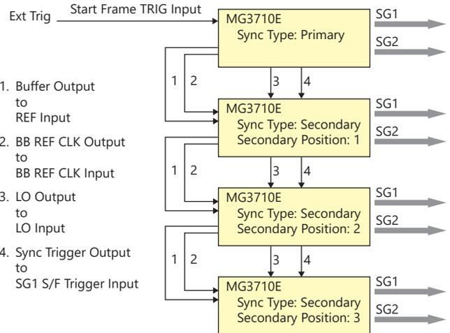
Note: MG3710E-017 is not required when synchronizing the local signal and baseband clock of SG1 (1stRF) and SG2 (2ndRF) installed in one MG3710E unit.
