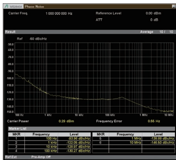
Phase Noise Measurement Low Phase Noise Performance MS2840A-066 Off 1 GHz Measurement Frequency, Preamp Off
