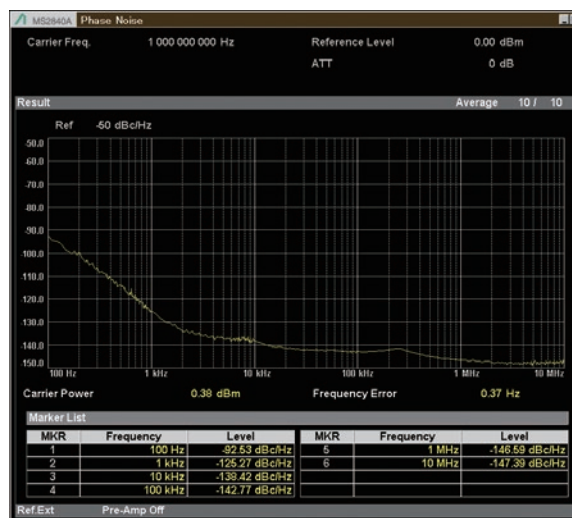
Phase Noise Measurement Low Phase Noise Performance MS2840A-066 On 1 GHz Measurement Frequency, Preamp Off
