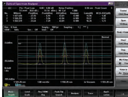
Example of Opt. Amp (Multi-channel) Analysis Function Measurement
