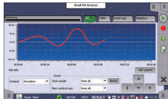
Phase Error Measurement by MU100090B
