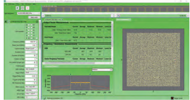
WLAN 11be TX Measurement using CombiView
