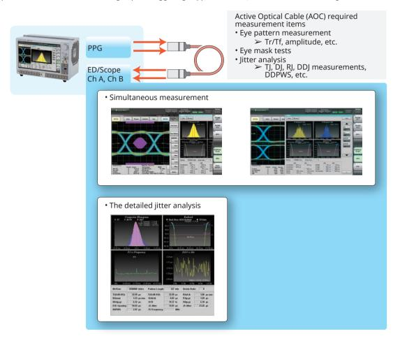
Simultaneous Eye pattern measurement, Eye mask test and jitter analysis
