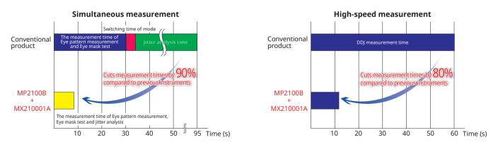
Typical values when capturing 106 samples at 10.3125 Gbit/s bit rate with PRBS15 test pattern at single-lane and back-to-back measurements
