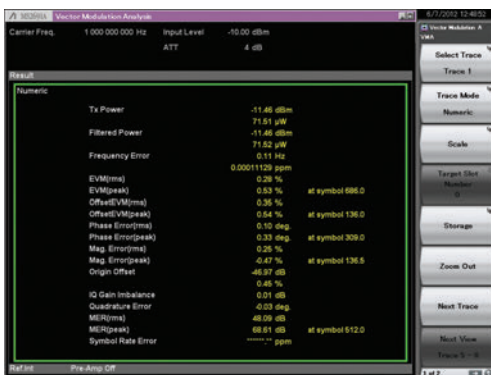
Modulation method: O-QPSK example
