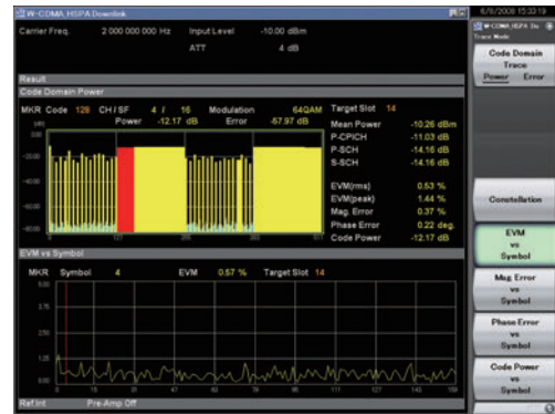
Code Domain (Vector Error vs. Symbol)
