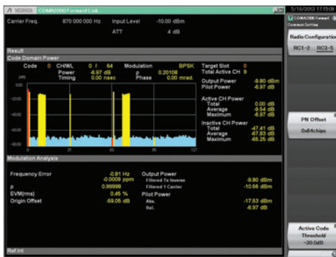
Code Domain Screen: CDMA2000 Forward Link
