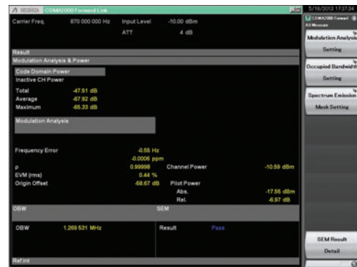
All Measure Screen: CDMA2000 Forward Link
