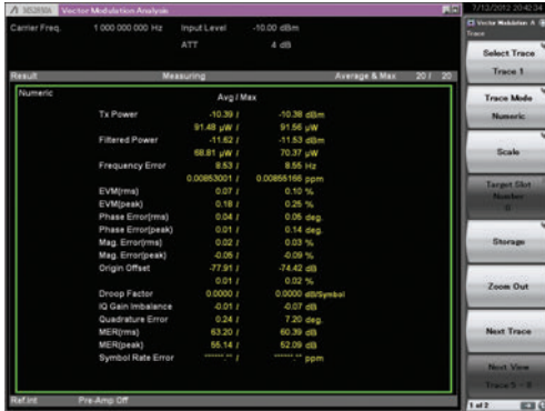
Modulation method: π/4DQPSK example
