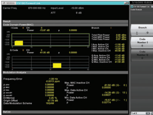
Code Domain Power Screen: EV-DO Forward Link
