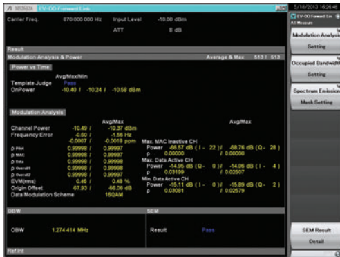
All Measure Screen: EV-DO Forward Link
