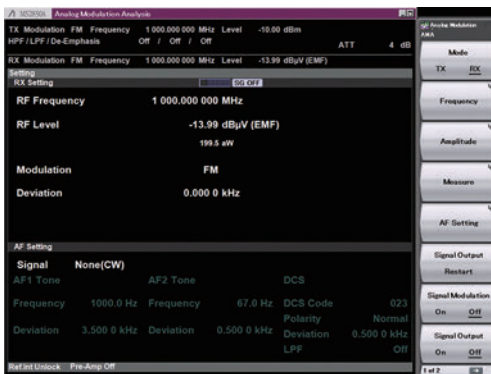
Example of RF Output Measurement Screen (with Analog Signal Generator)
