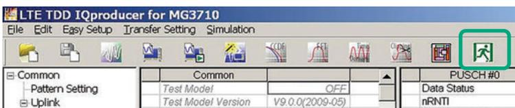
Displays Frame Structure screen for confirming channel allocation status and power of each OFDM Symbol
