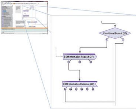
The flowchart based test design environment allows engineers at all levels of expertise to create tests quickly by dragging and connecting signaling blocks to define the test flow. Test parameters default to typical sensible values and can easily be adjusted using intuitive parameter dialog boxes.
